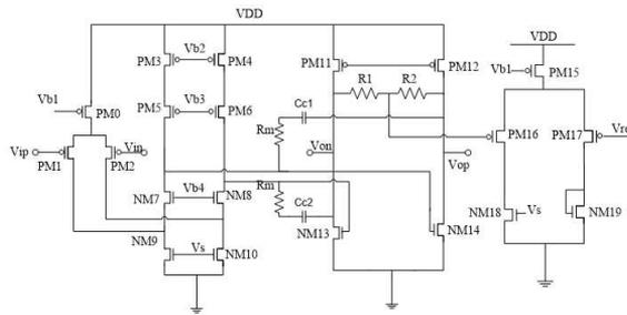
Fig. 2. The full differential operational amplifier circuit diagram
